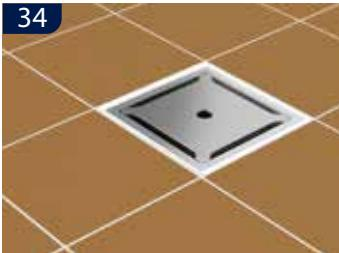
**UK** Insert water trap and filter basket. Install the grating, and the installation is complete. If a gas-tight cover is used, the O-ring should be lubricated with silicone grease before assembly.
