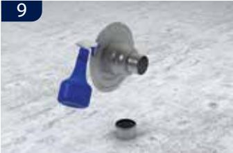
**(UK)** Wipe the outlet with a cloth and apply lubricant to the outlet for easy assembly.
